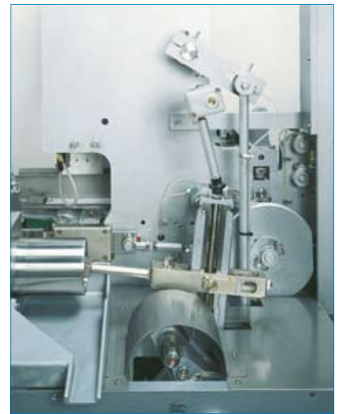
Drive of dosing station
